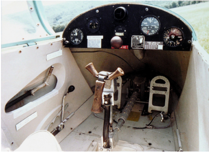
Figure 5: An early version of the hand control system.
