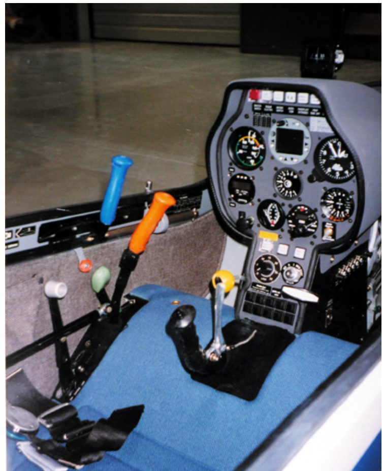
Figure 6: A later version of the hand control system in Bruce's self launch glider.
